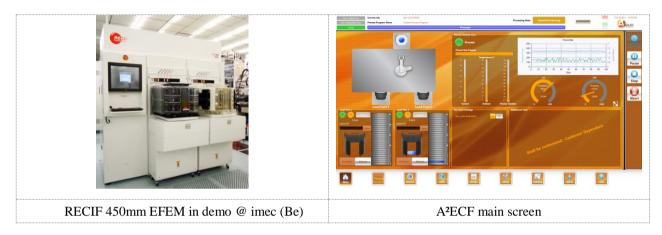
The Agileo Automation team employed 3 days to customize the robot drivers for the A<sup>2</sup>ECF solution to be able to control the RECIF 450mm/300mm EFEM. A<sup>2</sup>ECF is an equipment automation software solution that supports major EFEM platforms and delivers process and alarm management, recipe management, SEMI E95 compliant graphical user interface, and customizable schedulers with graphical representation.
